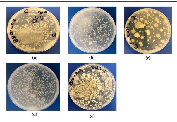
Fig. 7 Microbial growth on agar plate of soil for a untreated soil; b nutrients only; c cementation solution only; d biostimulation; e bioaugmentation
