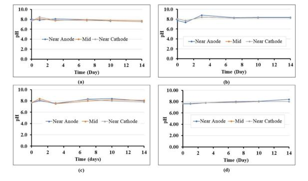
Fig. 5 pH changes in soil chamber during EK treatments, next to the electrolyte chambers and in the mid-point of soil sample: a nutrients only; b cementation solution only; c biostimulation; d bioaugmenta-
