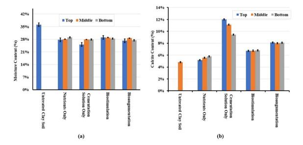
**Fig.9** a Moisture content of the soil sample (top, middle, and bottom of the sample) before and after treatment. **b**  $CaCO_3$  content of the soil before and after treatment
