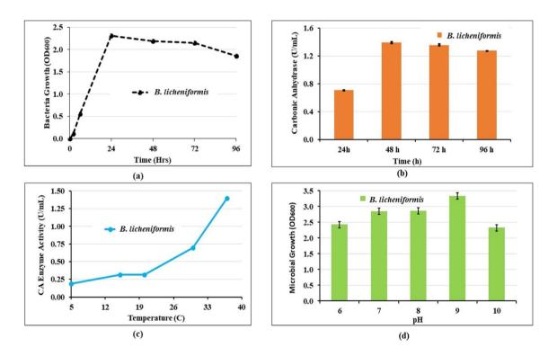
Fig. 3 Optimal growth characteristics of *B. licheniformis* isolated from the site used for bioaugmentation case: **a** microbial growth; **b** carbonic anhydrase (CA) enzyme production; **c** temperature; **d** pH
