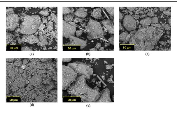
Fig. 10 Scanning electron microscope micrograph for a untreated soil, b nutrients only, c cementation solution only, d biostimulation, and e bioaugmentation
