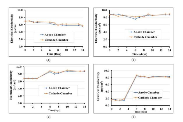
Fig. 6 Electrical conductivity changes of the anode and cathode chambers during various treatment procedures: **a** nutrients only; **b** cementation solution only; **c** biostimulation; **d** bioaugmentation using
